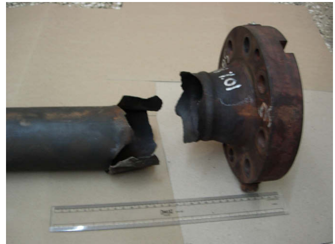
Fig. 2. The failed pipeline showing circumferential fracture and excessive thinning at the location of fracture.
